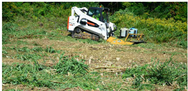
Wet blade mower applies herbicide as blade cuts vegetation.
