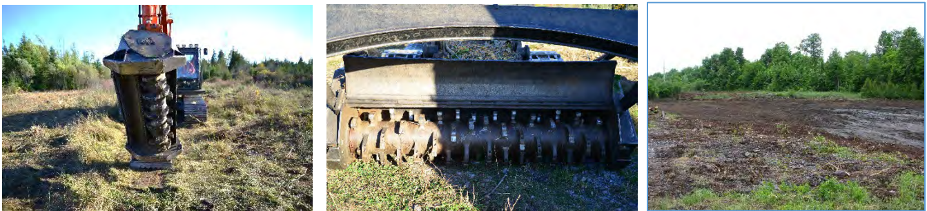
Crushers / grinders can be mounted on a number of vehicles and will cut vegetation and mix cut debris into soil & subsoil.
